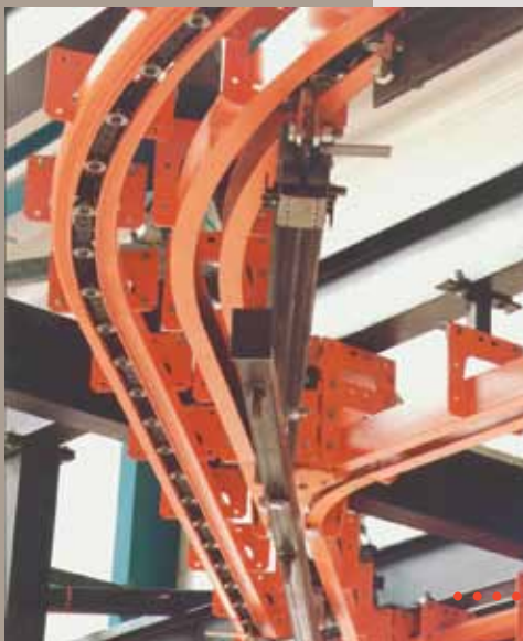
Switch in T4 P&F system
